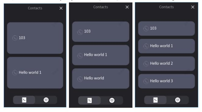
2) If added indoor station quantity is more than 5 (include 5), the user will show as contact list. Or you can also switch to keypad mode to input room number manually.
