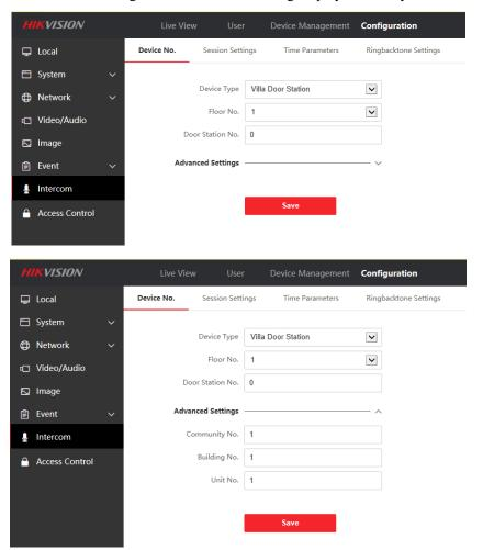
6. Support doorphone mode, when this function is enabled, the door station will no longer actively synchronize the information of the indoor station
