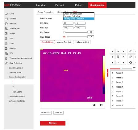
Using deep learning algorithm to detect vessels, which can realize ship flow detection, dredger detection and fishing ship detection.
