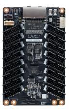
DS-DR32H-16 is a universal receiving card launched by Hikvision. A single card can load up to 512×512 pixels (HikLCT needs to be V5.3.1 and above), 14Bit+, light-by-light chromaticity correction, and RGB independent Gamma adjustment. , 3D and other functions to improve the screen display effect and enhance the user experience.
