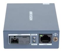
DS-3D501T-A is a gigabit single-mode single-fiber fiber optical transceiver developed by Hikvision. It provides one 10/100/1000 Mbps self-adaptive RJ45 port and one 1000 Mbps SC fiber optical port, and can achieve high-speed and lossless transmission of data signals over a maximum of 20 km transmission distance.
