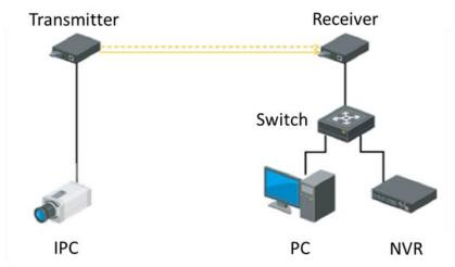
Application 2: IPCs Connected to Fiber Optical Transceiver (Transmitter) via a Switch
