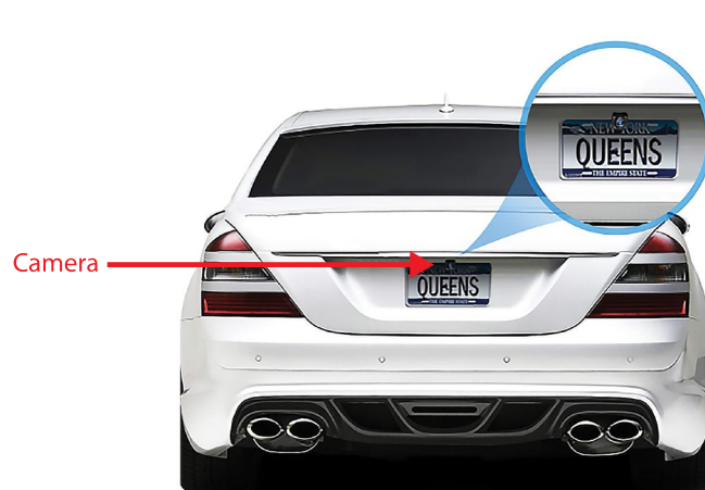
Figure 8, Rear Camera Exterior Placement
