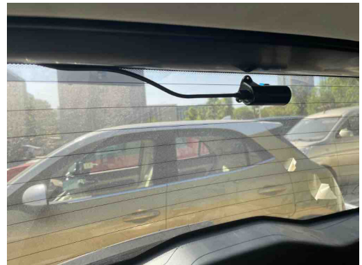
Figure 11, Rear Camera Interior Placement on Rear Windshield (Option 2)
