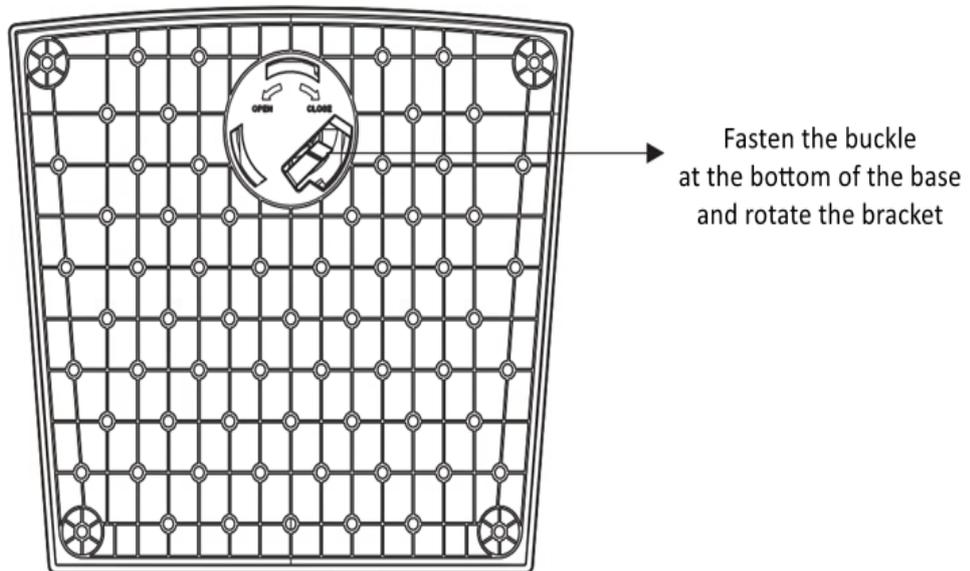
Figure 2-6 Remove the Bracket from the Square Base
