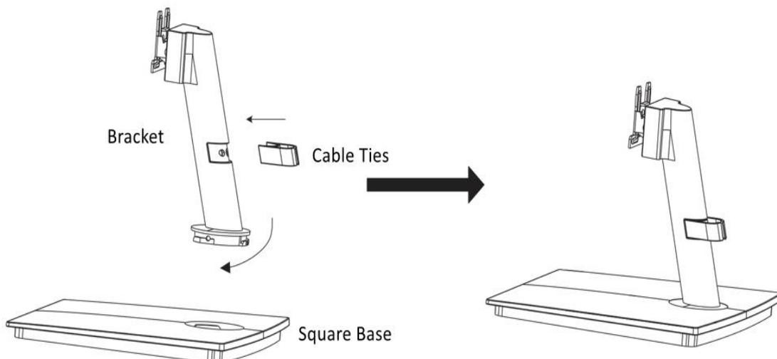
Figure 2-2 Fix the Bracket with the Square Base
