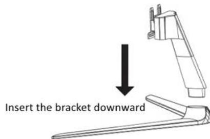
Figure 2-8 Install the Bracket
