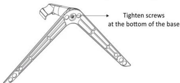
Figure 2-9 Tighten Screws
