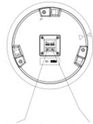
Red wire clamp is for positive pole. Black wire clamp is for negative pole.
