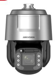
Hikvision 4 MP  $32 \times$  Network IR Speed Dome adopts 1/1.8" progressive scan CMOS chip. With the  $32 \times$  optical zoom lens, the camera offers more details over expansive areas.
