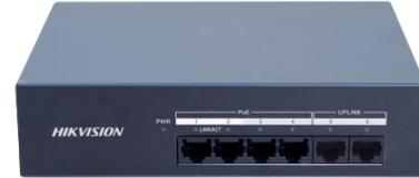
DS-XS06G-P provides four 10/100/1000 Mbps PoE RJ45 ports and two 10/100/1000 Mbps RJ45 ports, with up to 30 W output power for a single port and up to 35 W PoE output power for the whole device. Capable of intelligently identifying powered devices, DS-XS06G-P is plug-and-play, and simple in use.
